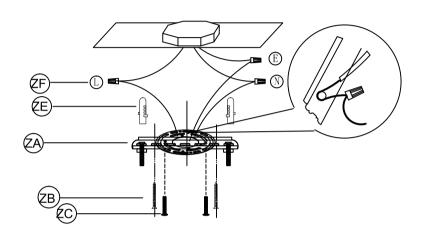
Drill two holes on the ceiling and put the plastic anchor screw(ZE) into the holes(If the wall is wood made, this step can be ignored);
