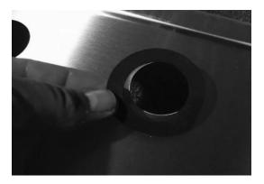
**Step five** – Feed of the (hot and cold) lines through the (faucet hole 1 3/8 inch in diameter)
